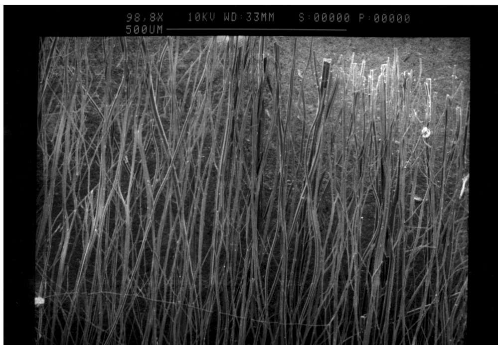
Figure 1 Photograph demonstrating the alignment of magnetite fibres.
